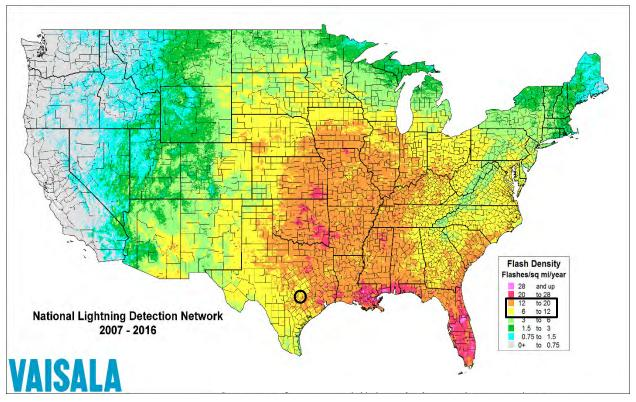
Figure 11-1. Lightning Flash Density, 2007-2016
