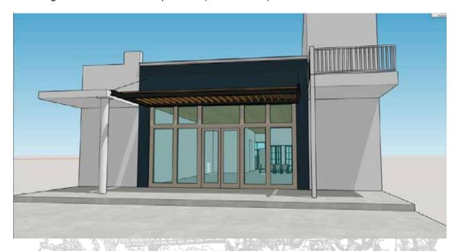
The new awning would be a steel flat awing with painted steel channels at the perimeter and stained wood infill including exposed joists. The awning will be connected with steel rod tiebacks to the stone façade (Attachment 6).
