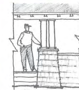
Short paired boxed columns on top of shingled, tapered pedestal
